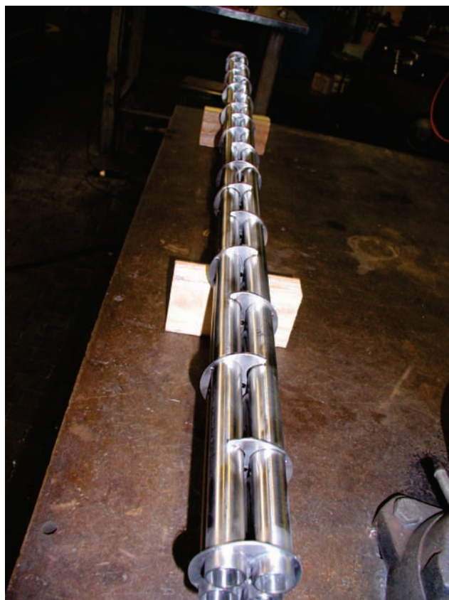
Figure 6. Internal reaction tubes and extra-tubular baffles for the Quad four-tube trickle-bed reactor are shown. For each tube, diameter is 1 in., and the length is 72 in.
